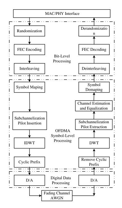
Figure 2: Block Diagram of proposed Wavelet based mobile WiMAX (IEEE 802.16e OFDMA-PHY)
