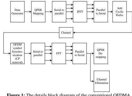
**Figure 1:** The details block diagram of the conventional OFDMA engine for WiMAX model.
