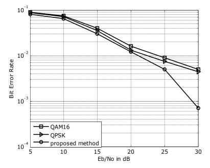
**Figure 3:** BER performance versus Eb/N0 for ordinary OFDMA using QAM16 and proposed wavelet based OFDMA scheme.
